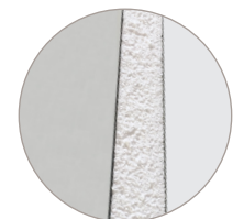
POLYSTYRENE INSULATED CORE
