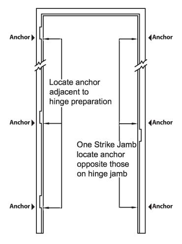
You will have been furnished with one(or more) of the illustrated types of loose stud wall anchors necessary for the installation of the UL listed Fire door frame provided on this job.
