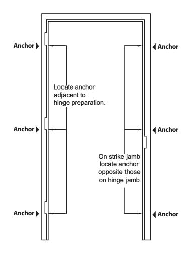
You will have been furnished with one (or more) of the illustrated types of loose masonry wall anchors necessary for the installation of the UL listed Fire Door Frame provided on this job.
