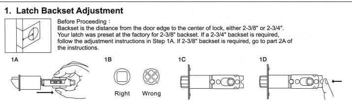
1A. If 2-3/4" backset is required, pull spindle cam all the way to the right edge of the adjusting hole.
