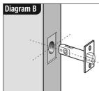
Fit the latch support post on the inside of the front plate, in outer hole side A for a left hand hung door and in outer hole B for a right hand hung door. (See diagram C).
