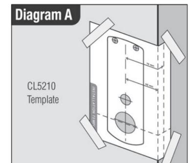
2. Keeping the drill level and straight, drill a 25mm (1") hole in the center of the door edge to accept the latch. Put the latch into the hole and holding it square to the door edge, draw around the faceplate. Starting with the top and bottom cuts, chisel a rebate to allow the latch faceplate to fit flush with the door edge. Remove the latch.
