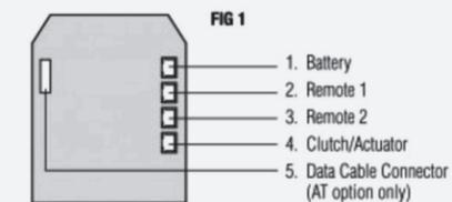
REM 1 is for connection to a reception desk push button or a door intercom system. Pressing the button will cause the Blue LED to flash on the lock and release the lock for the pre-set time.
