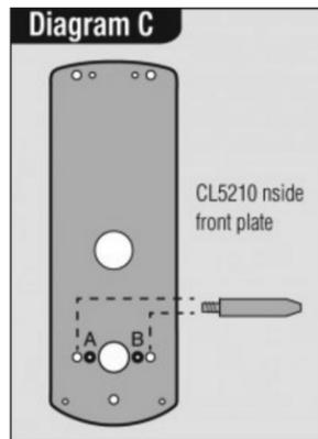
7. Screw the cable tube into the front plate, passing the cable through the tube. For doors less than 45mm (1 3/4") thick screw the tube all the way to the end of the thread. For doors more than 45mm (1 3/4") leave an appropriate amount of thread showing.
