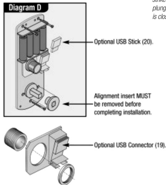
13. Check that the spindle turns freely, and the latch retracts and projects smoothly, with the alignment insert in place. If it is tight, loosen the fixing bolts slightly and adjust the position of the fixing plate until the spindle will turn freely. Tighten the fixing bolts. Test the spindle again. Do not over-tighten the bolts as this may cause the door to distort and affect the lock function. REMOVE THE ALIGNMENT INSERT.
