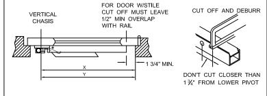
C. DREPRESS ARM INTO RAIL OPENING AND SLIDE RAIL ONTO CHASIS. LEVEL RAIL AND FASTEN CHASIS AND MOUNTING PLATE.
